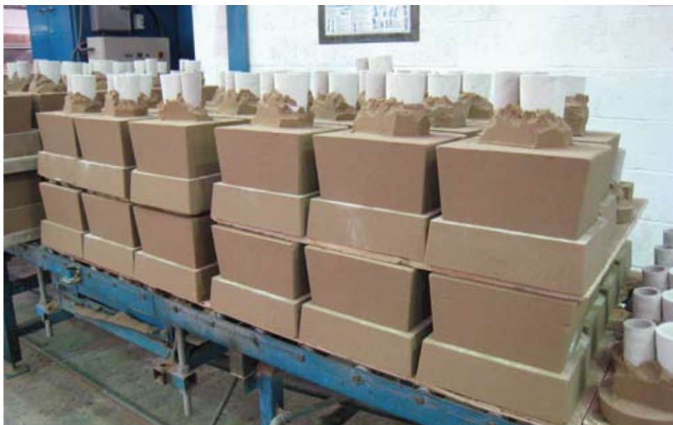
Examples of moulds and cores in production at the foundry
